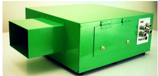
Figure 2. Portable LIBS prototype for industrial on-line applications. Left: schematic view of the different components Right: photograph of LIBS prototype
