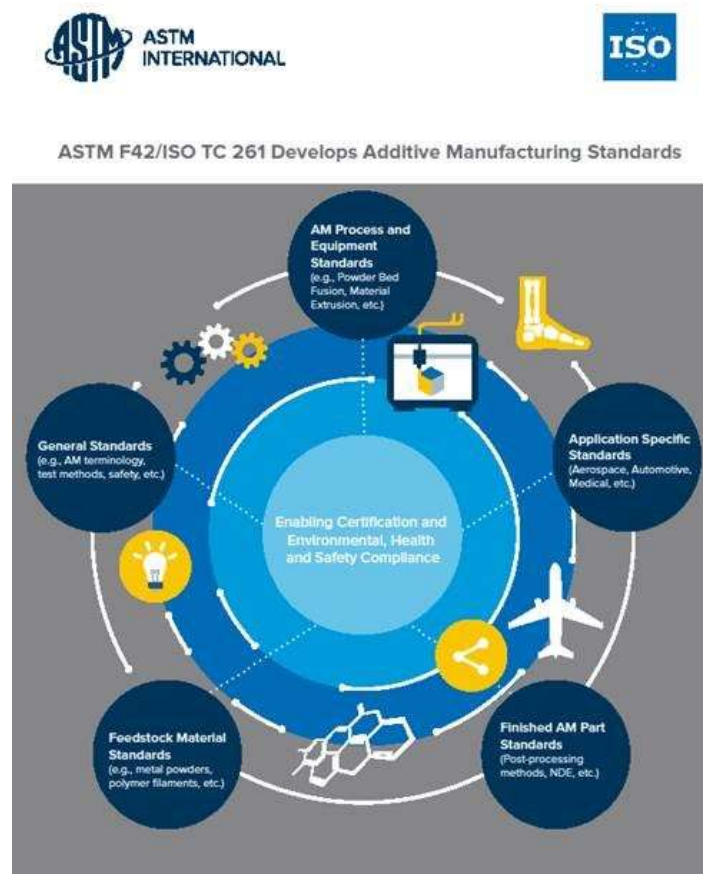
Figure 2 An overview of different areas for AM standardization from ASTM F42/ISO TC 261 5
