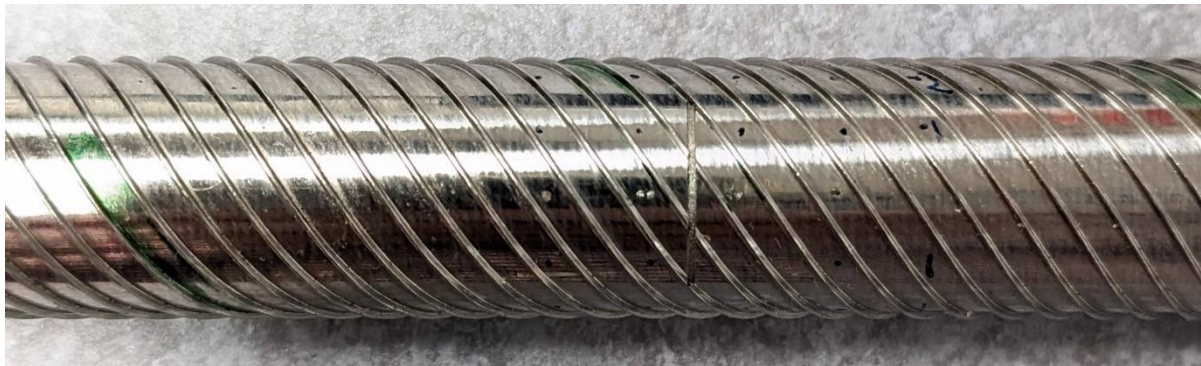
Figure 1. Photograph of an AGR fuel rod showing the ribbed pattern and a notch across the ribs.
