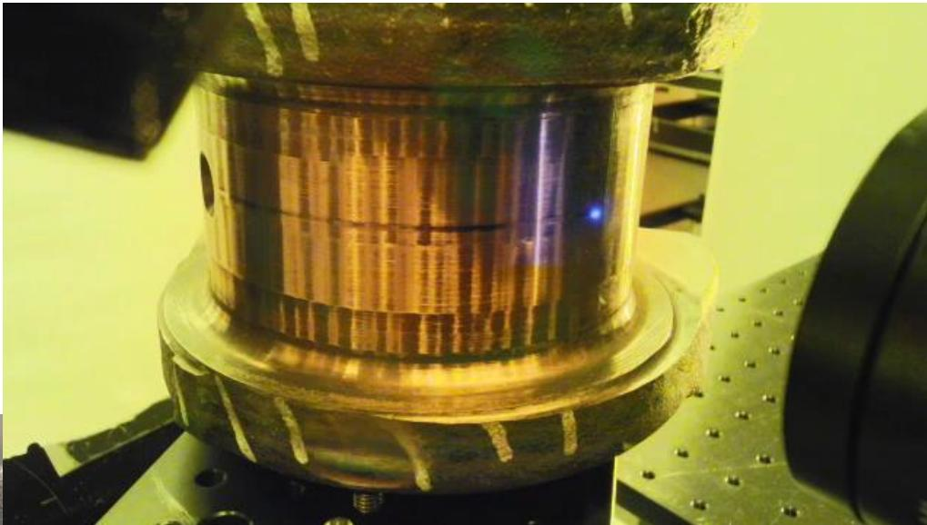
One measurement = hole edge to hole edge, ~350 degrees
