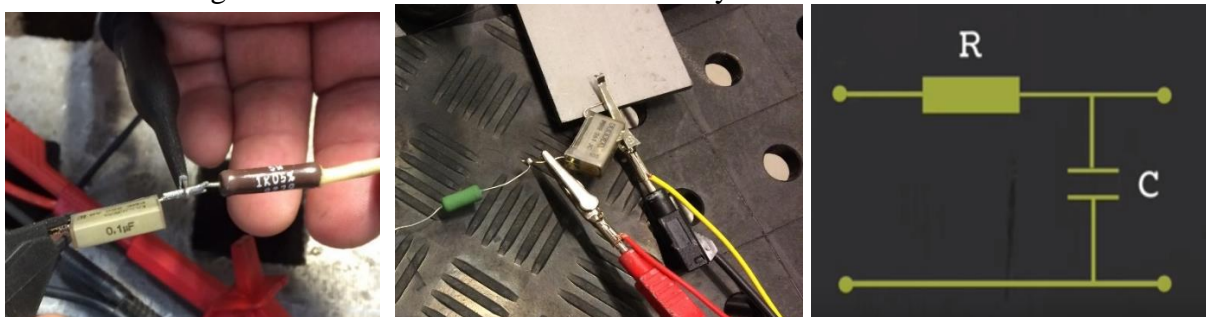
Figure 3: The photos and the schematic illustration show a low pass filter with a cut-off frequency of approximately 1.6 kHz ( f_c = \frac{1}{2\pi RC} ). The voltage is measured over the capacitor.
