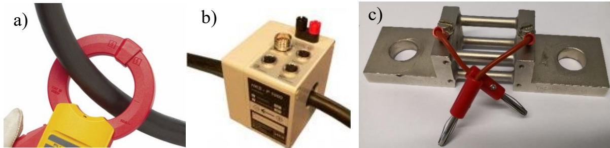
Figure 1: Sensors for current measurements: a) clamp meter b) Hall element sensor and c) current shunt resistor
